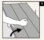
When a plank is locked, it is not possible to take it up by hand. Separate the whole row by carefully lifting up and slightly knocking just above the joint. Fold up and release the whole long side.
