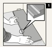
First plank, first row. Start in a left corner with tongue side facing wall and long groove side directly up against straight edge. Spread adhesive enough to cover one plank width. Use only as much adhesive as can be used during manufacturer's open time of adhesive.
