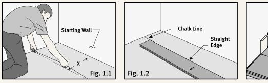
Using starting wall as reference, snap chalk line on subfloor at distance X from wall as shown in Fig. 1.1. Align straight edge with chalk line and secure to subfloor.
