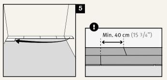
Start the second row with the off-cut from the first row. **①** Note! It must be at least 16" (40 cm) between the short end joints of the planks.
