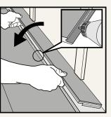
Remove the locking element/hook according to the picture. Use white PVAc glue to connect the planks. Press- place wedges between the glued plank and the wall.
