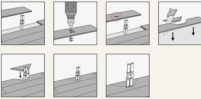
Mark the center point of the tubes on the plank. Drill holes 1" (20 mm) bigger than the tube diameter (if gap distance is chosen to be  $\frac{1}{2}$ " (10 mm)). Cut according to the picture. Put white glue and replace the floor pieces. Cover the holes with pipe collars or fill with a joint sealer.
