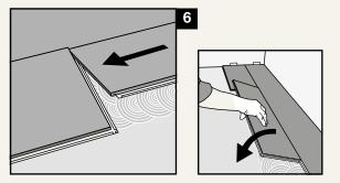
Second plank, second row. Place the plank gently and tight to the short end of the previous plank. Fold the plank down in a single movement. Make sure the plank are tight against each other. Press down the plank.
