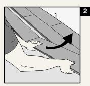
After the whole long side is released you can disassemble each plank by angling the short sides up vertically.
