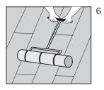
The floor must be rolled with a 50-Kg roller, every 30 minutes, and upon completion of installation, to ensure that the tiles are firmly bedded into the adhesive
